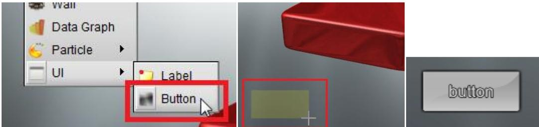
3. Double click on the button, open the "UI Node Setup", we can use any image to replace the current one. And you can set the text on the button, if you don't need the text, just delete it.
